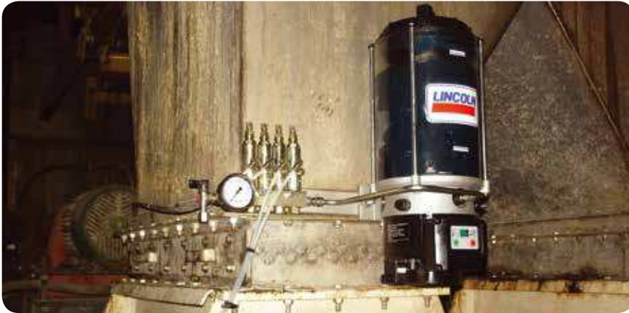
This Centro-Matic automatic electric pump and injectors are lubricating bearings in a very abrasive and dusty environment.
