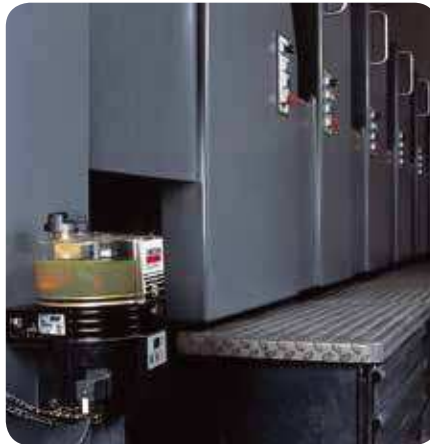
This Lincoln Quicklub QLS oil system virtually eliminates manual lubrication on bearings and gears for this printing press. Lubricating on-the-fly improves productivity.
